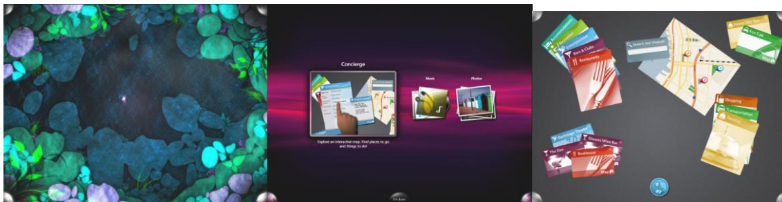
Figure 3-4: Microsoft Surface first orients Launcher based on which access point has been touched (towards either long side of the screen) in the attract application. Then, any application launched will also be oriented in the same way, by default.
